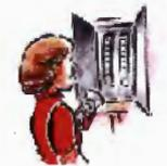
The electricity goes to the **service panel** in your basement or garage, where breakers or fuses protect the wires inside your house from being overloaded.
